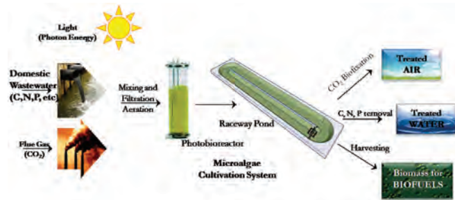
Schematic diagram of microalgae based waste water treatment plant
