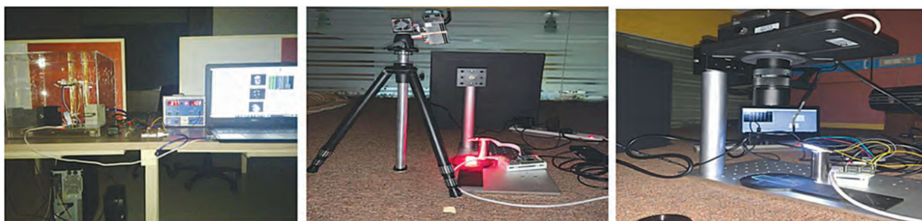
Facilities available under Microarray platform technologies for in-situ, on-chip protein expression classifier for biomarker discovery. (L-R) Integrated System Prototype, Fluorescence acquisition & analysis system and Ultra low light intensity imaging system
